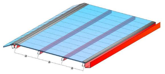
The loading table of **NEWLUX** PC Panels (below) has to be considered for safe load resistances while the distances (a) between the construction rafters of the roof or the wall are formed. Minimum slope of 12% is advised for roof applications.
