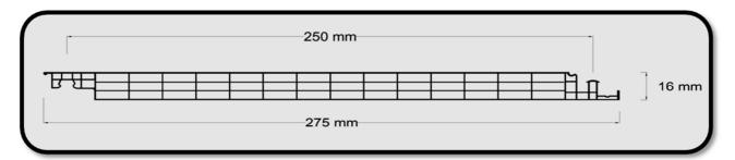
**NEWLUX** PC Modular Panels have 250 mm module width, 16 mm thickness, 4 walled body structure, high light transmission and thermal insulation. A hidden screw slot is used on the installation of **NEWLUX** PC panels, and lock into each other easily and safely by special side design. Through the **NEWLUX** connection detail, roof and wall lighting areas can be covered practically, safely and with continuous transparency against heat, wind and water without any connection accessories.
