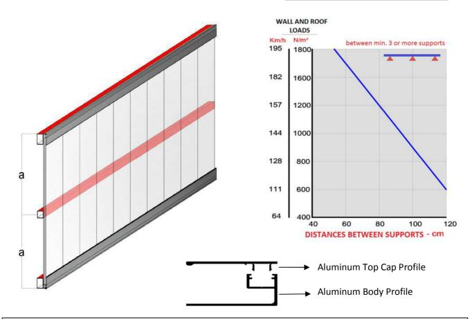
Before the application, both ends of the PC panels should be closed by adhesive tapes. An aluminum cap with a hidden screw and body profiles are needed for the installation of **NEWLUX** panels. EPDM gasket should be used to ensure application without water leakages. If requested, ventilation window systems for roof and wall that are compatible with **NEWLUX** are available. The system can be controlled through drives.
